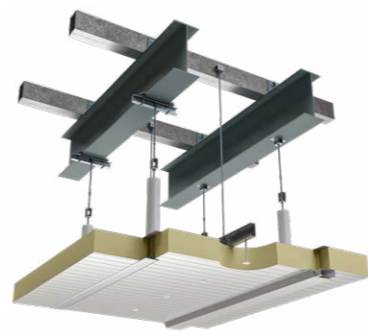
顶板吊挂系统 Top Panel Hanging System
